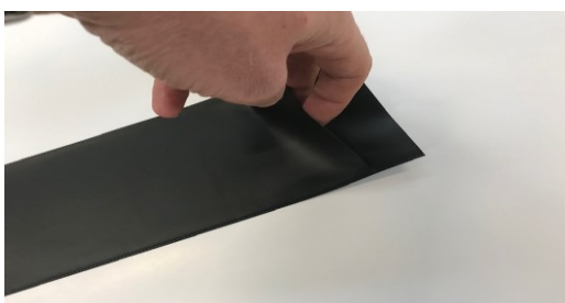
Super Flat cassette opening and a fold over light proof seal
