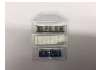
Example 10 FE EN indicator with 5.0mm wire spacing and 10mm wire length
