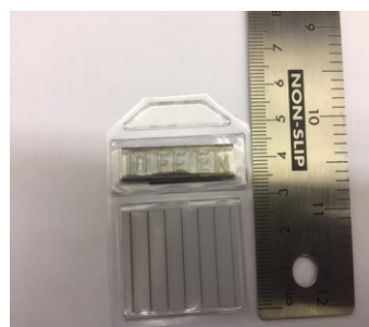
Example shown of 10 FE EN IQI with 5mm wire spacing and 25mm wire
