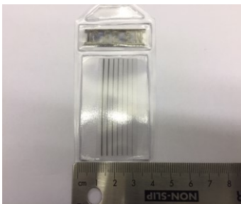
Example 10 FE EN indicator with 2.5mm wire spacing and 50mm wire length
