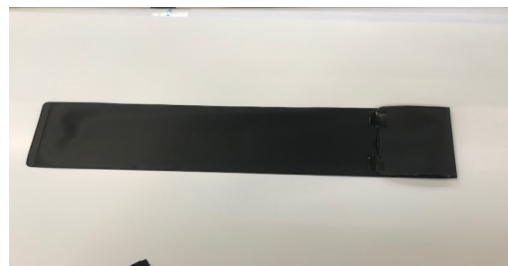
Super Flat cassette with light proof seal folded and secured with adhesive tape
